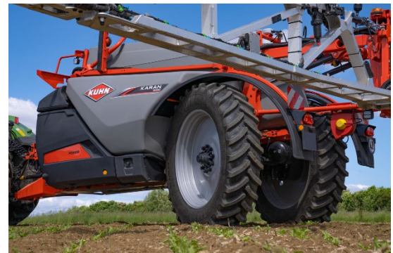
3. WITH ITS COMPACT DIMENSIONS AND FEATURES (ESPECIALLY THE STEERING AXLE), KARAN IS AN EXCEPTIONALLY MANOEUVRABLE SPRAYER
